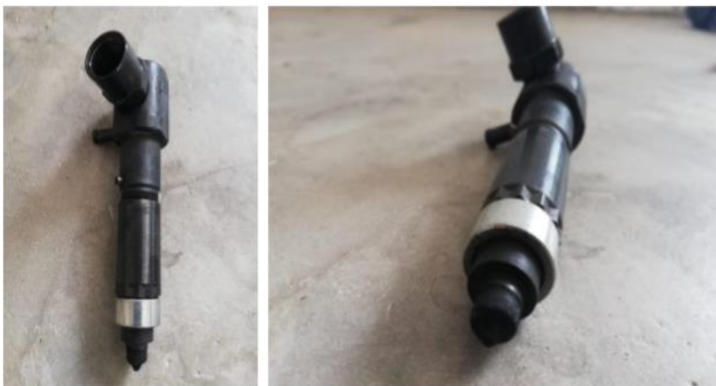
Figure 3 – Status of the injector nozzles of the Vonder GDV 5500 generator, after 2000 hours of operation with our BBL 100
