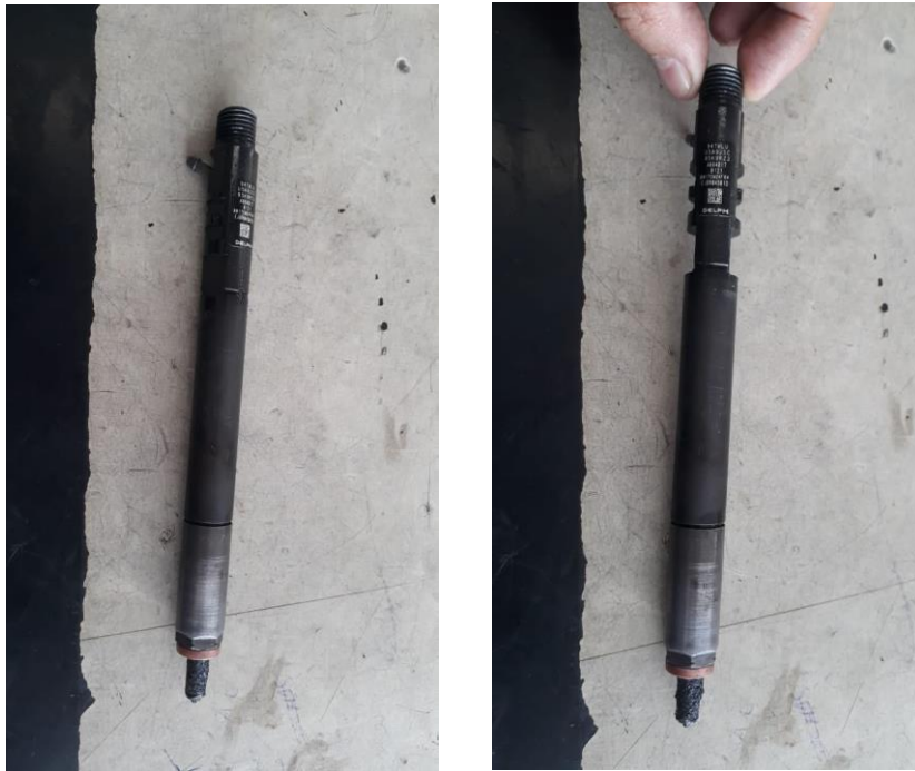
Figure 2. Images of the injector nozzle of the SsangYong Kyron 2.0 4x4 Diesel engine.
