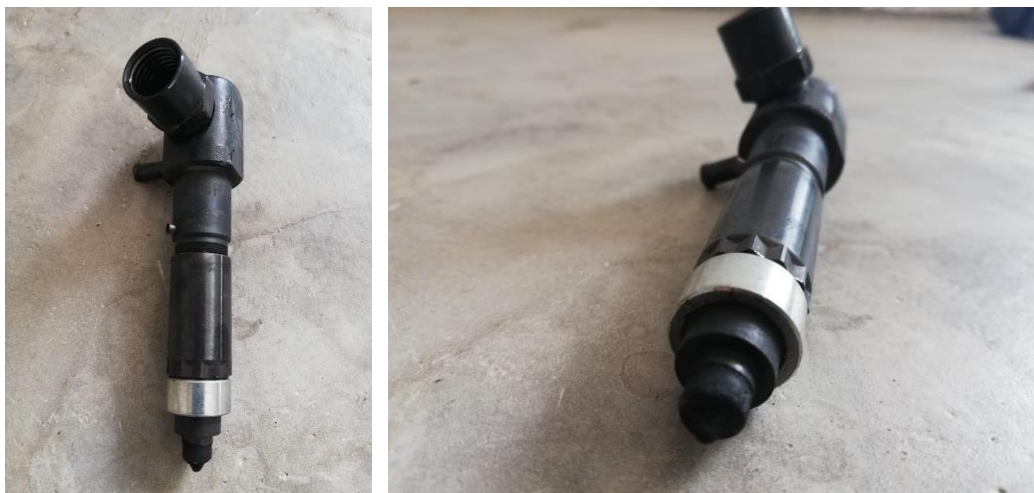
Figure 2. Images of the injector nozzle of the GDV 5500 Vonder Diesel Generator engine.
