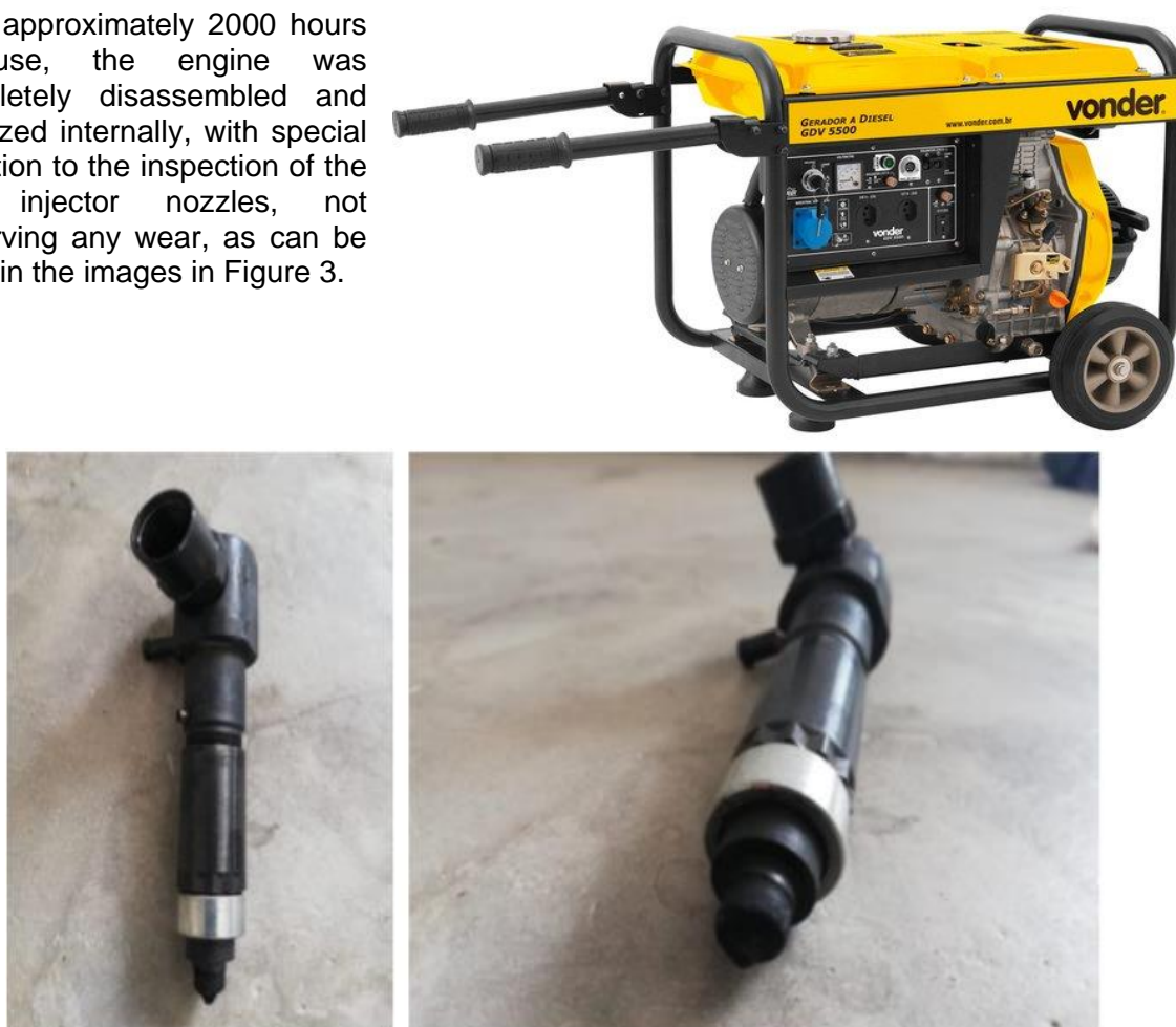
Figure 3 – Status of the injector nozzles of the Vonder GDV 5500 generator, after 2000 hours of operation with our BBL 100
