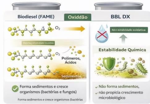
These phenomena lead, in a few months, to the **degradation of fuel quality**, with direct impacts on filters, pumps, injectors and tanks – an effect visually evidenced by the formation of sludge at the bottom of the container after short periods of storage.
