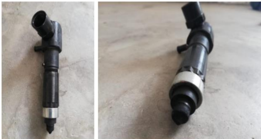
BLL DX 100 - Status of the injector nozzles of the Vonder GDV 5500 generator, after 2000 hours of operation
